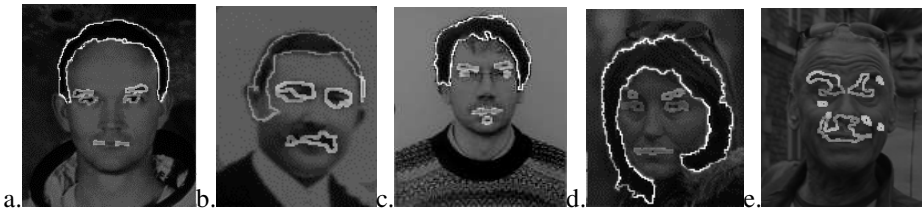
Fig.7. Interpretation of segmentation results of faces. Regions labelled as eyes, mouth and hair are shown by overlapping their edges with the original images.
