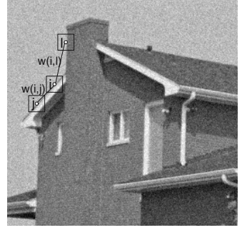
Fig. 1. Illustration of the window representation of pixels. w(i,j) is large because their neighbouring windows are similar. w(i,l) is much smaller.
